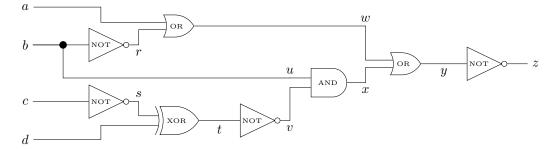
5.3.10 Compute the propositional formula  $\varphi$  represented by the following circuit. Furthermore, compute an equisatisfiable formula  $\varphi'$  using the Tseitin transformation.
