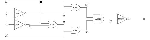
5.3.11 Compute the propositional formula  $\varphi$  represented by the following circuit. Furthermore, compute an equisatisfiable formula  $\varphi'$  using the Tseitin transformation.
